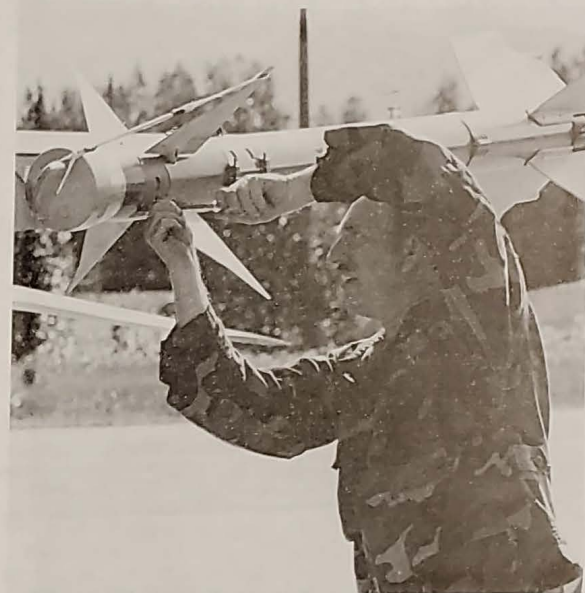
MSgt. Gary Seale, prepares an AIM-9 wingtip missile prior to flight. (U.S. Air Force photo)
